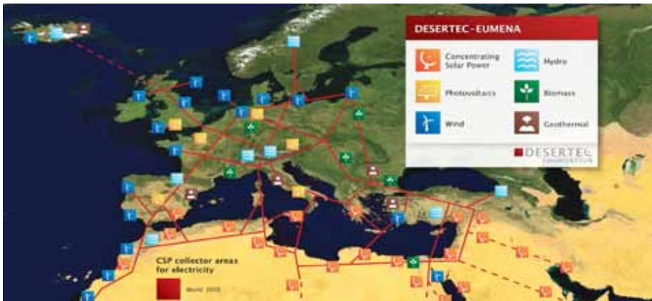
Figure 3 HVDC lines connecting the economic sites for harvesting renewable energies in EU and MENA. Estimated losses 3% for each 1000 km (Source: DESERTEC Foundation)
