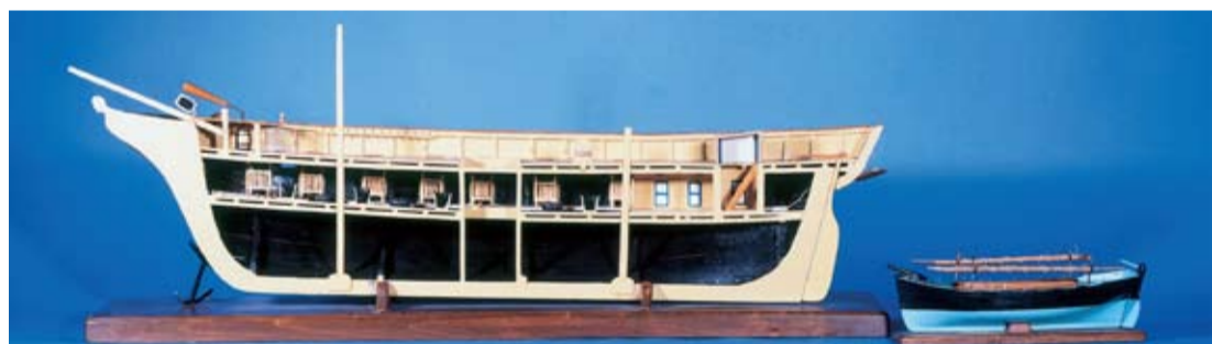
A section of a scale model of a fireship with a scapavia rowing boat in tow
