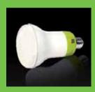
Like CFLs and LED lamps, the new ESL bulbs use a phosphor; however, one that does not absorb light at all, but absorbs electrons instead. Roughly speaking, ESLs are cathode-ray tubes repurposed as lamps. The electrons stream off a metal cathode plate and are pulled by an electric field toward an anode, a thin layer of metal on the backside of the phosphor.
