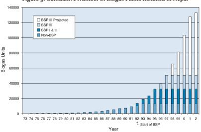
Figure 3: Cumulative Number of Biogas Plants Installed in Nepal
