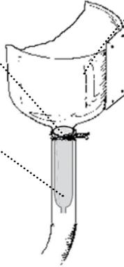
**You have to put the collection tank underground** and isolate it to prevent freezing during winter.
