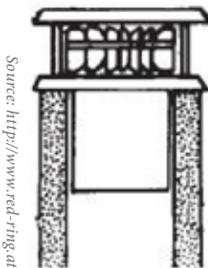
A wind driven or electric ventilator reduces the possibility of bad smell.
