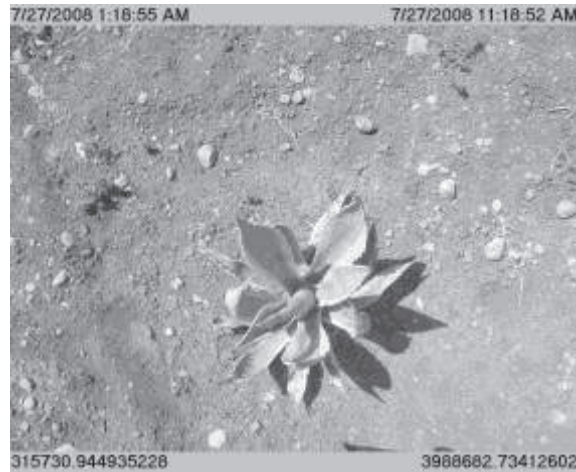
Figure 4. Collared image showing the date, local time and GMT of when the image was taken (top) and easting and northing coordinates of its exact location (bottom).
