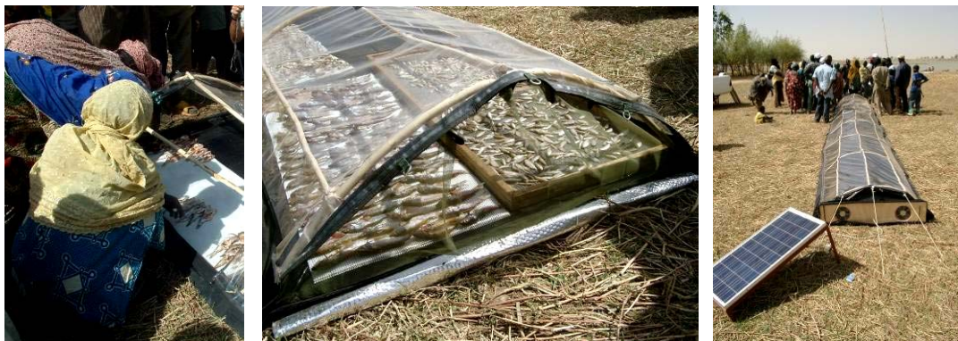
Figure 8. Testing a mobile USISS type dryer for fish at Dagawomina, Mali
