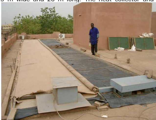
Figure 1. Present director of USISS with the double solar tunnel dryer (drying racks against the wall of the handling room).
