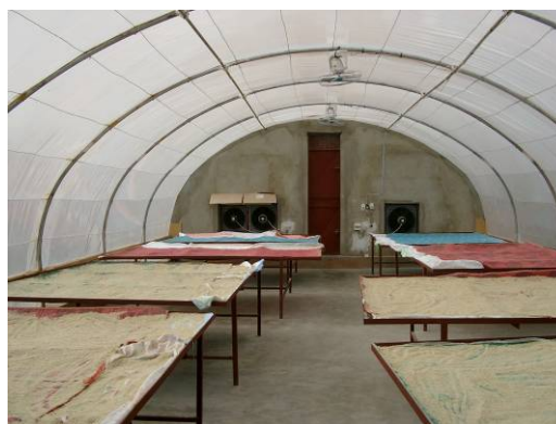
Figure 10 Greenhouse dryer for Fonio, Mali
