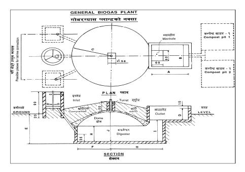
Figure-10 Drawing of Nepal GGC 2047 Biogas Plant
