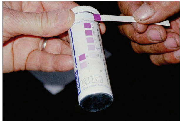
Example of a nitrate quick-test, this particular test showed the drinking water well had a level of nitrates exceeding 500 mg per liter (max. WHO level 50 mg/l).
