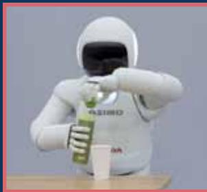
or run on two feet at speeds up to 6 kilometers per hour, climb up and down the stairs, and even dance. He can also adjust the length of his steps, body position, speed, and the direction in which he is stepping. ASIMO has arms and hands that can do things like turn on light switches, open doors, carry objects, and push carts.
