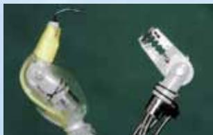
They worked together, creating a mini-robot that mimics the shape and movement of a crab's pincers. The robot is attached to an endoscope, with a small camera to provide visual feedback. It has the ability to go down a patient's throat and remove cancerous tissue by having the pincer hold the cancerous tissues, and then the hook slices them off, coagulating blood to stop any bleeding.
