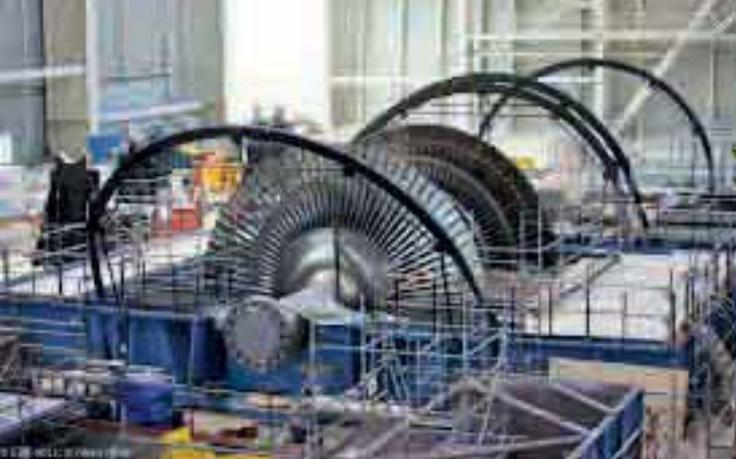
As is typical in all conventional thermal power stations, the heat is used to generate steam, which drives a steam turbine connected to a generator that produces electricity. Nuclear power plants are usually considered base load stations. This means that a very small amount of fuel can produce the target required amount of power; hence, fuel is a small part of the cost of production, while the major cost of production lies within the construction and operation of the facility itself.
