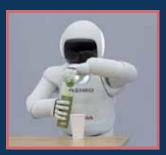
or run on two feet at speeds up to 6 kilometers per hour, climb up and down the stairs, and even dance. He can also adjust the length of his steps, body position, speed, and the direction in which he is stepping. ASIMO has arms and hands that can do things like turn on light switches, open doors, carry objects, and push carts.
