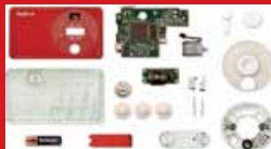
The camera looks a bit like a science experiment, which is the point. The back cover is transparent, providing a view of the gadget's gearbox, dynamo, processor chip and circuits, enabling young users to better understand the relationships among the different components. The front cover of the plastic prototype comes in colors inspired by M&M candy!
