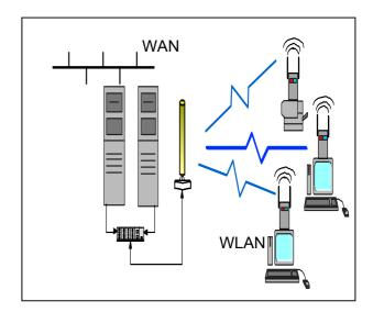
Here, a LAN is connected to another network using a wireless connection. The two transmitters/ receivers function as a point-to-point connection, but the distance is limited. Since the antennas do not need to point towards each other, devices can be placed anywhere within the range of the transmitter/receiver.
