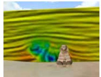
The LIC plane visualized both the air field shape and the pressure values using colors
