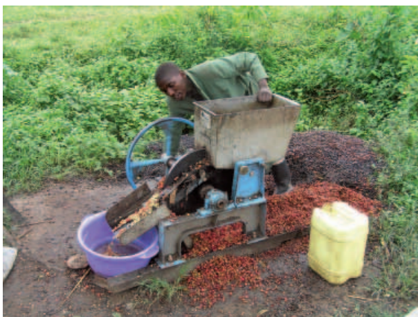
Smallholder farmer in Rwanda producing fully washed coffee using a hand pulper
